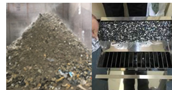
Research on optimization of ASR recovered resin recycling process. Left photo is ASR, right photo is resin recovered from ASR
