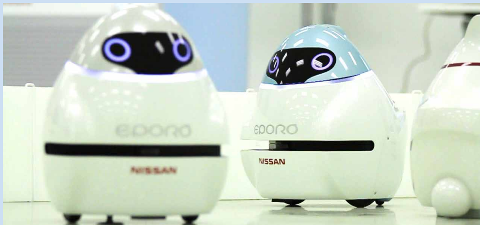
EPORO robots developed to study collision avoidance.
